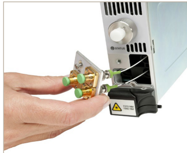
Step-by-step example of opening the front panel door to maintain the launch connectors
