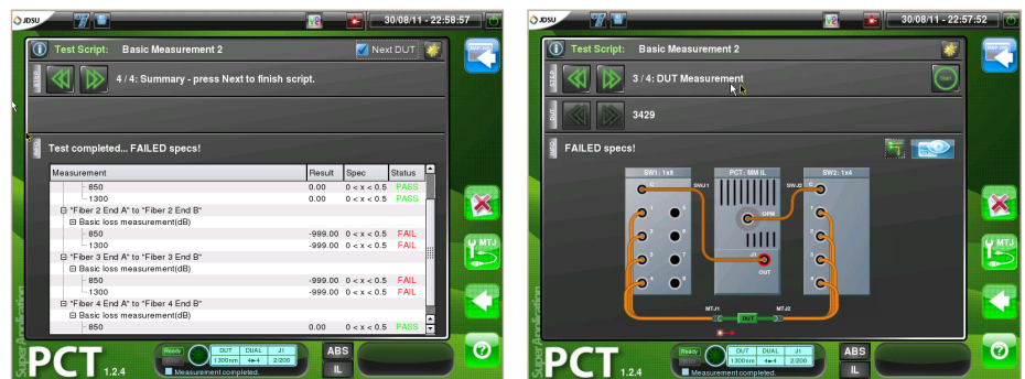
Screen shots from the onboard script mode for production testing
