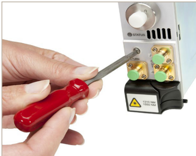
Step-by-step example of opening the front panel door to maintain the launch connectors
