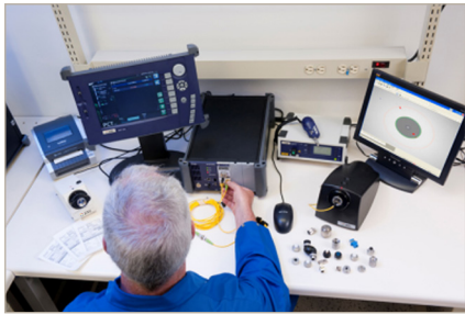
Operator leveraging the IL/ORL test solution alongside connector inspections
