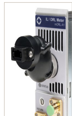
The JDSU AC990 attached to the front panel of an mORL module with an MPO power meter adaptor
